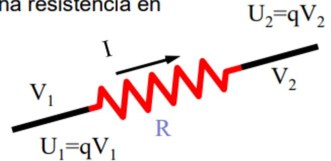
$$\Delta U = q\Delta V = q(V_2 - V_1) = qIR$$
